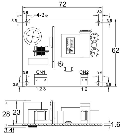
AC input connector (CN1): Molex5273 series or equivalent
