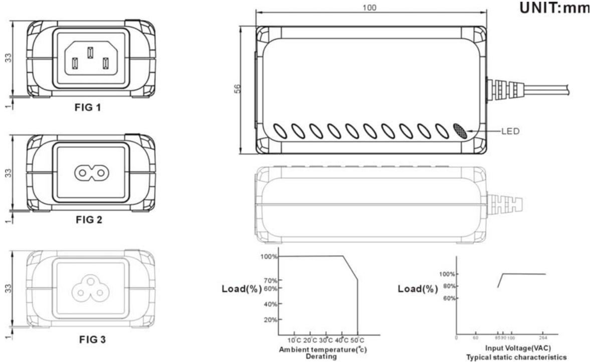
X=A=IEC-320-C14 (FIG1) or B=IEC-320-C8 (FIG2) or C=IEC-320-C6 (FIG3)
